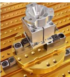
material cost. These modular clamps and stops are ground to the same height as our Large Modular **Pitbull**® Clamp (page 13) providing even greater versatility.
