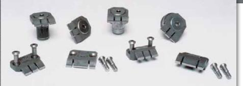
These low profile cam action clamps and stops have a holding force of 880 lbs. (3900N.) and have fingers that push the workpiece down before clamping, even on castings that have negative draft!
