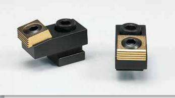
This clamp is like the Compact Toe Clamp, only it is designed to be used in the T-slots of machine tables. It provides 4,000 lbs. (17800 N) positive down force while maintaining a low profile. The hardened steel clamping element has both a smooth surface for machined workpieces and a serrated clamping surface for rougher work.
