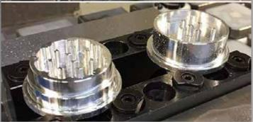
VersaGrip<sup>™</sup>, as the name implies, offers the versatility of clamping standard vise work as well as providing a solution for difficult applications that would normally require fixturing or machining soft-jaws. By simply replacing your current jaws with the VersaGrip<sup>™</sup> system you can securely hold odd shaped parts while machining at speeds and feeds you never thought possible.
