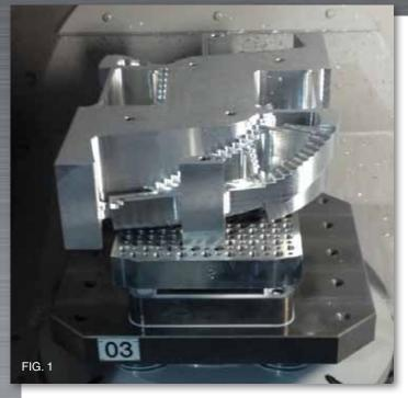
The Mitee-Bite Loc-Down® System was designed to be a programmer's and operator's dream for quickly and easily securing small to large aerospace parts. Its compact design allows for tighter pattern on grid plates compared to other options in the marketplace saving material cost on expensive aerospace alloys.
