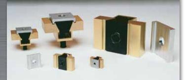
The compact Mitee-Bite Uniforce® clamp is available with extra material on the clamping jaws so it can be machined to conform to the shape of your workpiece enabling you to fixture unusual applications easily. The specially designed steel wedge spreads the clamping force uniformly on both sides of the 7075-T6 aluminum channel.
