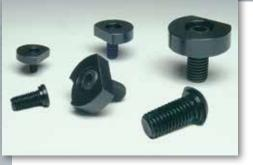
These clamps, with the machinable steel washers, provide more flexibility for holding round or unusual shaped parts. Parts can be held directly to the fixture plate surface or elevated for through drilling. A special screw is provided with each package to hold the washer in the proper place during machining.
