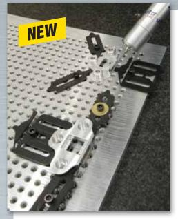
The Spring-Loc<sup>™</sup> is an extremely low profile (.072") adjustable clamp capable of producing approximately 10 lbs. of clamping pressure depending on how much the flex arm is compressed in the locked position. The center slot allows 360° positioning. The back end of the Spring-Loc<sup>™</sup> is "V" shaped allowing customers to run parts in series for engraving, laser etching and provides a simple and quick method for locating and holding parts for CMM and Vision Systems.
