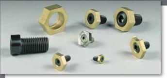
The cam action MITEE-BITE Fixture Clamp is made up of two simple components: a hardened steel socket cap screw with an offset head and a brass hexagonal washer.
