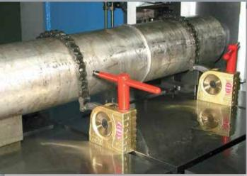
The Mono-Bloc Chain Clamp is a simple and rapid workholding solution for a wide array of applications.
