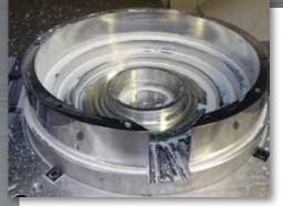
The popular Pitbull<sup>®</sup> Fixture Clamp is now available in a machinable version. The clamp has positive down force and a very low gripping profile, reducing material cost and number of operations.
