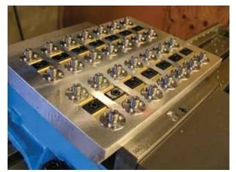
Fixtured with Mitee-Bite Machinable Uniforce® Clamps
