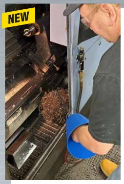
SAFETY! A work related accident can happen very easily. Always use a chip hook to clear away annoying chips and empty the chip trays on your machines. The new design provides a simple, solid method to remove chips from hazardous and hard to reach areas. Second generation chip hook features a large cone which offers protection for the entire hand, single or double-handed handles available. Bright blue color guarantees high visibility and wooden handle ensures a firm grip.
