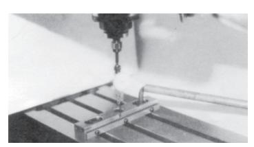
1. Indicate the master clamping bar to the table slots and tighten the bolts to 60 ft lbs. Hex key extension may be necessary to tighten properly.
