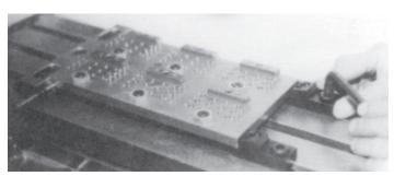
4. Tighten both Mitee-Bite cam clamps. **CAUTION!** Over tightening of clamps could cause master clamping bar to move. In extreme situations the use of Mitee-Bite T-slot Clamps (not shown) can correct this, simply tighten T-slot Clamps against the master rail on the opposite side.
