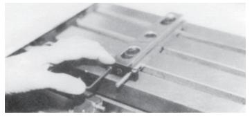
2. Mount adjustable stop on preferred end of master clamping bar with screws provided.
