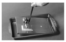
Use air or water to cool, being careful to prevent water from going between subplate and workpiece while hot.
