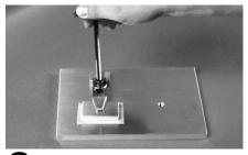
2 In some instances a weight or clamp with light pressure may be used to locate part. NOTE: Over large thin workpieces use a top plate for even pressure.
