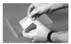
Place the Mitee-Grip paper on the subplate leaving a 1/4" border on all sides of the part
