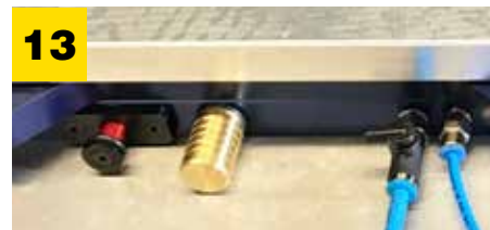
Visual red indicator identifying vacuum off.
