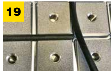
Close up of recommended method of sealing chamber. Place end of Gasket approximately 25% into perpendicular slot. Cut with scissors for clean straight end.
