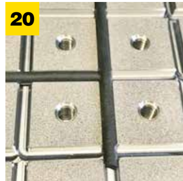
Take care in adjusting Gasket to obtain best seal possible. Ensure Gasket is in contact with bottom of slot, check entire length for gaps using flashlight. Vacuum Grease (PN 45094) and Installation Tool included to ease installation.
