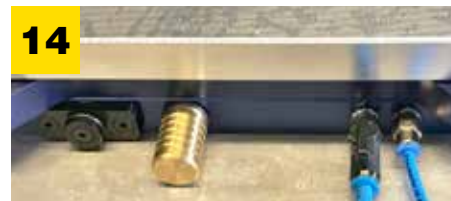
Visual indicator identifying vacuum on.
