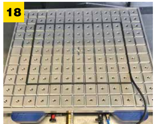
Sealing Gasket installed in channel.
