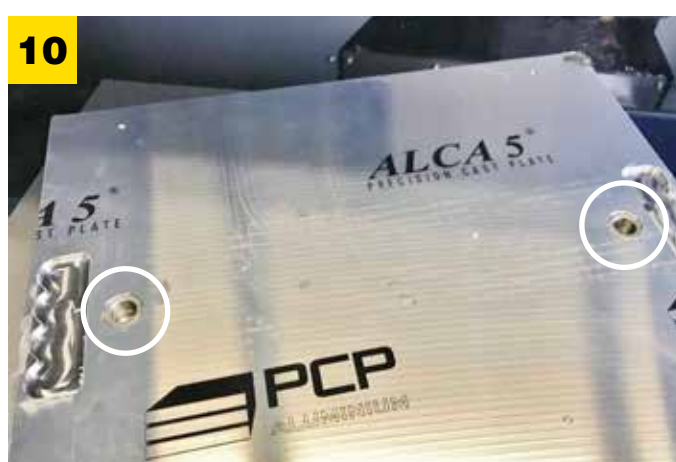
Bottom of Blank Pallet (PN 45130 or 45135) identifying precision drill bushings and grip points. \varnothing = 10.630"/270mm .
