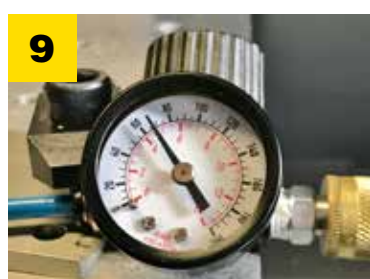
Adjust air pressure to 70-75 PSI or 5 bar.
