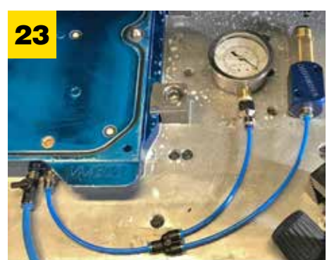
Open supply valve and check indicator and gauge for proper pressure. If using LPTS we recommend mounting on backside of machine and adjust LPTS using gauge.
