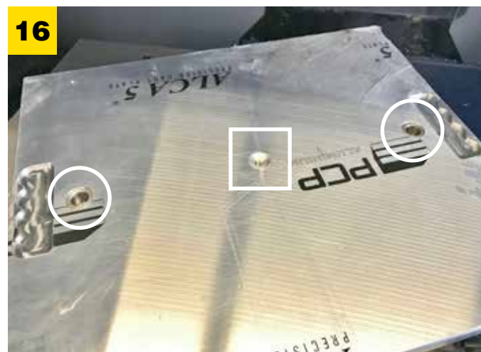
Bottom of Vacuum Pallet identifying through hole in center and both precision drill bushing. \varnothing = 10.630"/270mm .
