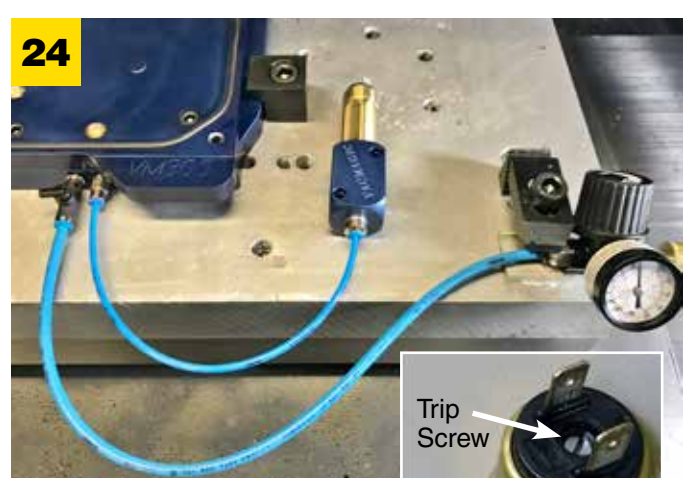
This Vacuum System can be configured to stop machining functions immediately. Have a qualified technician connect Low Pressure Trip Switch to the FEED HOLD circuit. This LPTS has an adjustment screw between the two prongs allowing you to set the "trip" pressure.
