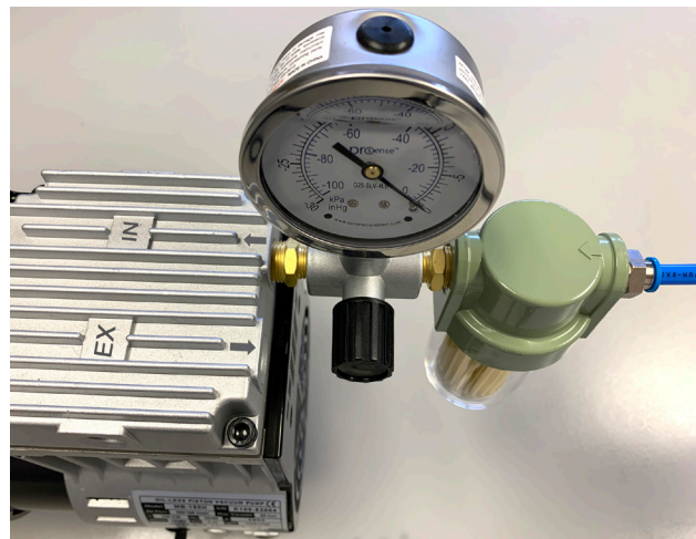
Vacuum Port set-up
