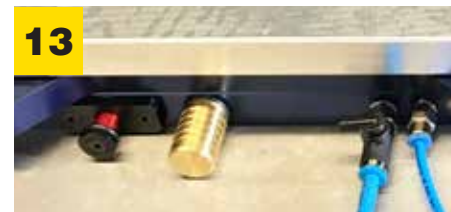
Visual red indicator identifying vacuum off.
