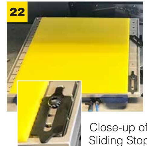
Workpiece positioned against Sliding Stops (PN 44200).
