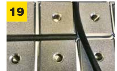
Close up of recommended method of sealing chamber. Place end of Gasket approximately 25% into perpendicular slot. Cut with scissors for clean straight end.
