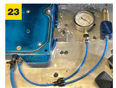
Open supply valve and check indicator and gauge for proper pressure. If using LPTS we recommend mounting on backside of machine and adjust LPTS using gauge.
