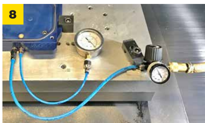
Assemble Regulator and attach with 6mm tubing to Supply Valve. Using 4mm tubing, attach Vacuum Gauge and/or Low Pressure Trip Switch fitting (located next to Supply Valve).
