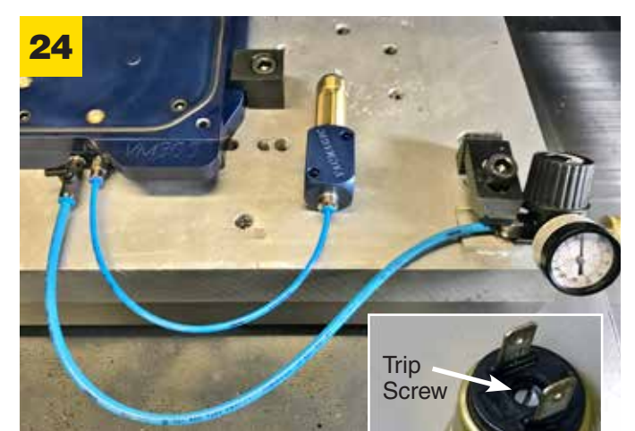
This Vacuum System can be configured to stop machining functions immediately. Have a qualified technician connect Low Pressure Trip Switch to the FEED HOLD circuit. This LPTS has an adjustment screw between the two prongs allowing you to set the "trip" pressure.
