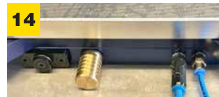
Visual indicator identifying vacuum on.
