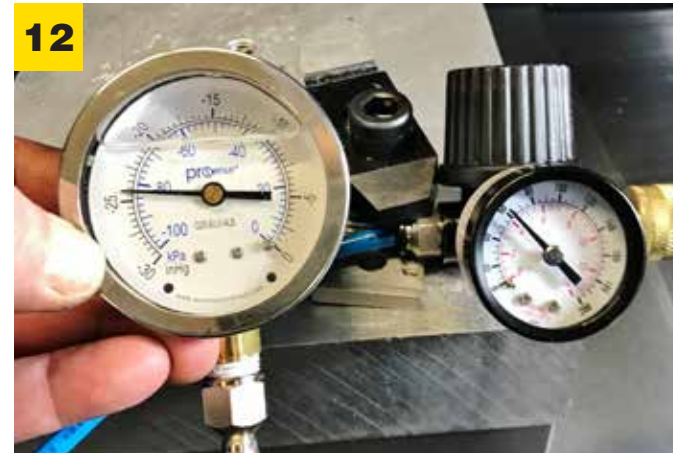
With Blank Pallet installed adjust air pressure with regulator until highest vacuum is obtained.
