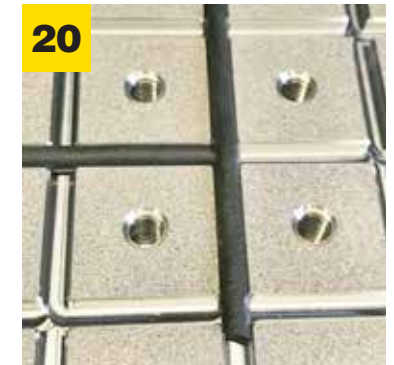
Ensure Gasket is in contact with bottom of slot, check entire length for gaps using flashlight.
