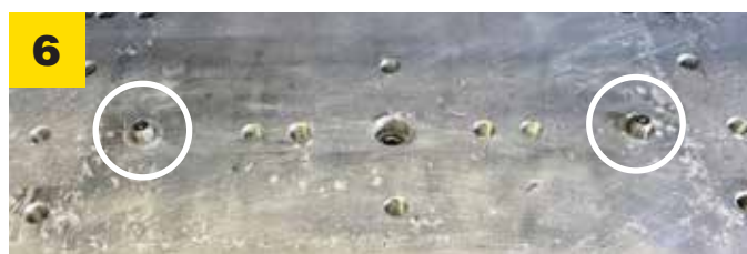
Machine platform with diamond taper pins allows quick and precise installation and removal of your tooling. Base Unit placed on these pins for location and rigidity.
